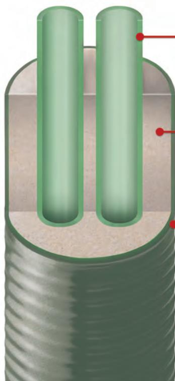
**PIPE:** Oxygen-barrier Central PEX® is a high-density, cross-link pipe, rated for 180°F at 100 psi. It is compatible with standard PEX insert fittings that cost much less than competitors' compression fittings. PEX lines are marked to easily identify supply and return lines.
